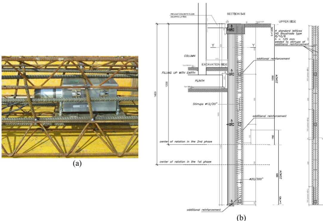
Figure 5: Prototype of embedded sensor module (a) and embedded sensor layout (b).
