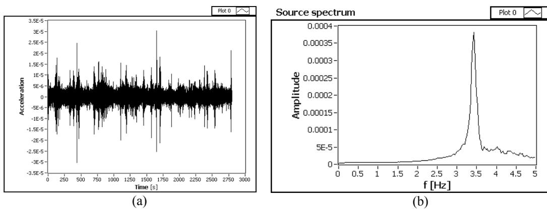
Figure 6: Sample record - acceleration in g - (a) and identified source spectrum (b).
