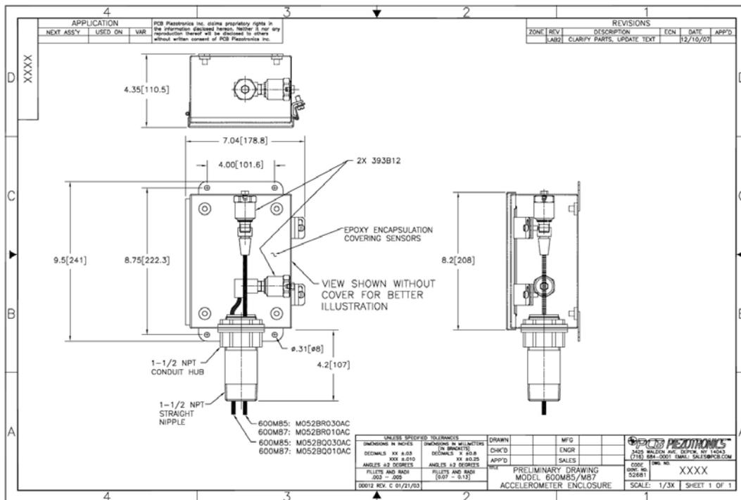
Figure 2: Scheme of developed sensor module (courtesy of PCB Piezotronics Inc.).
