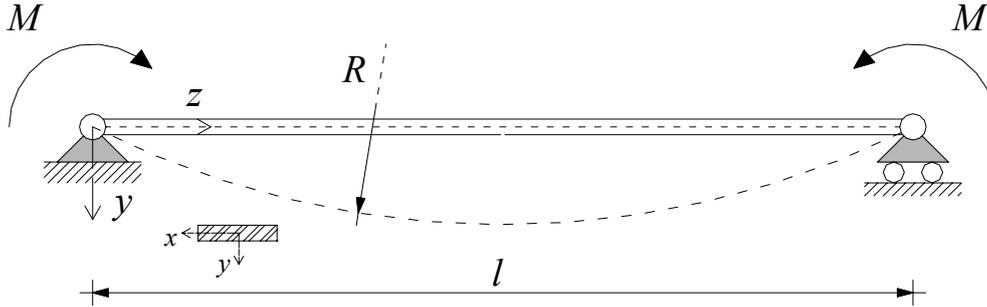
Figure 2: Schematic representation of bending of a beam of length  $l$  under the action of a couple of moments  $M$  applied at its ends.
