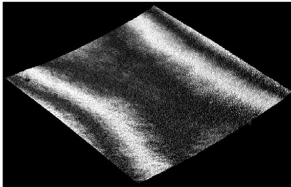
Figure 5: Deformation of the crystal surface when bent by the holder. The crystal is diced at  $\theta = 35.26^\circ$ . A saddle deformation is visible thanks to interference fringes.
