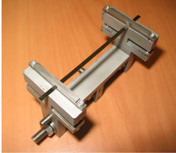
Figure 4: A silicon strip-like crystal bent by a mechanical holder.
