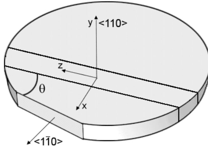
Figure 3: Silicon crystals are diced from a (110) wafer. The length of 70 mm is achieved at several angles  $\theta$  with respect to the wafer's flat. The Y axis is always the  $\langle 110 \rangle$  direction, while  $x$  and  $z$  vary as function of  $\theta$ .
