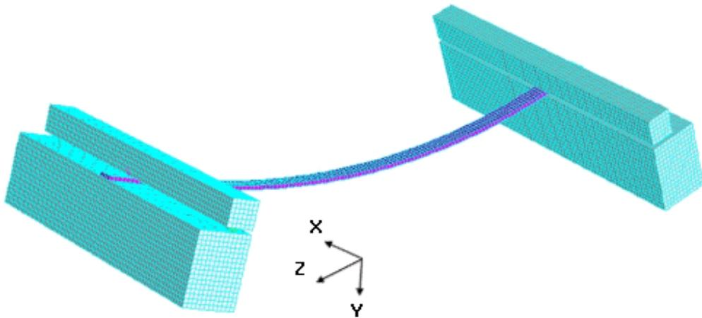
Figure 7: Mesh of a silicon strip mounted on the holder jaws for FEM. The strip ( $2 \times 0.5 \text{ mm}^2$ ) is simulated by 528 bricks elements, whereas 36496 bricks elements model the holder supports.
