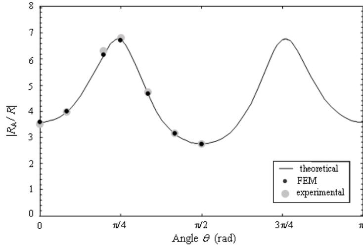
Figure 6: Ratio  $|R_A/R|$  as function of  $\theta$  (for its definition see Fig. 3). Experimental data are compared with FEM simulation and with the model. The figure shows that the ratio  $|R_A/R|$  is direction dependent as expected from a crystal.
