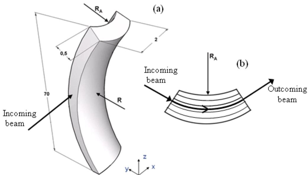
Figure 1: (a) Sketch of a bent silicon strip for channeling experiments (quotes are expressed in mm). (b) Cross-section of the crystal; the incoming particles are captured by the potential of atomic planes and the beam is being deflected.
