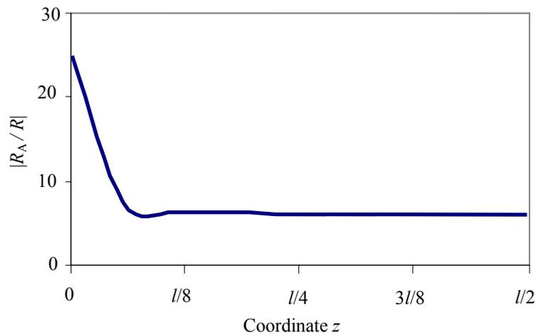
Figure 8: FEM-simulated values of  $|R_A/R|$  along the length of a bent crystal cut at  $\theta = 35.26^\circ$  and  $R_A = 12$  m. The numerical values largely agree with the theoretical prediction  $|R_A/R| = 6.2$  except for a small region of the crystal close to the jaws of the holder.
