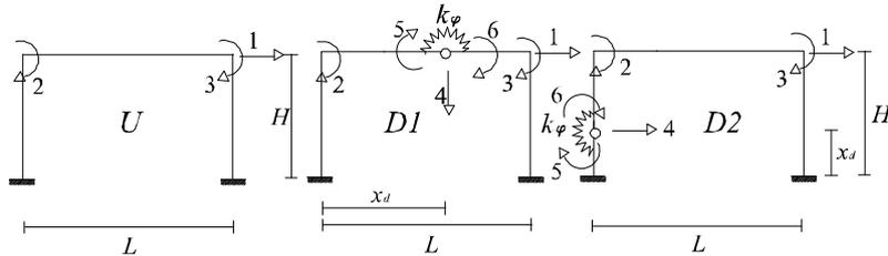
Figure 2 Undamaged and damaged models
