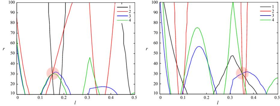
Figure 5 Curves  $r_i(l_j)$  for damage located at  $l=0.15$  a) and at  $l=0.35$  b),  $r=30$ .
