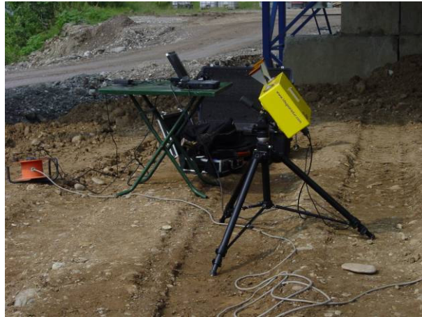
Figure 1: View of the microwave interferometer (IDS, model IBIS-S ).
