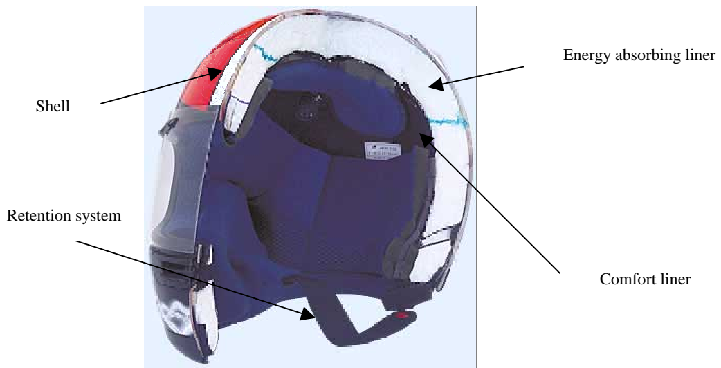
Figure 1: Structural components of a conventional helmet.
