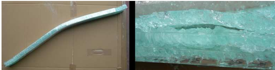
Figure 10: Glass element at the end of compression measurement.
