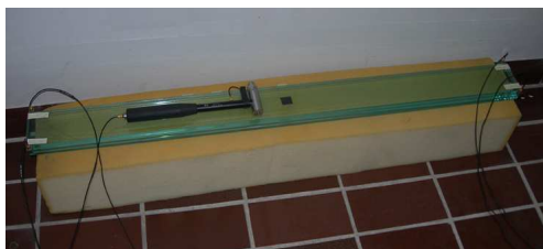
Figure 11: Configuration of vibration measurement.
