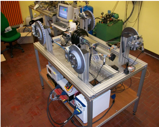
Figure 5: ABS/ESC HIL test bench
