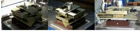
Figure 1: Bidirectional active mass damper with stroke stops and actuator saturation.
