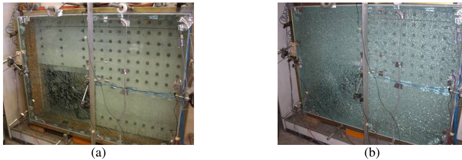
Figure 3: Post-glass-breakage tests. Partially broken panel (a) and completely broken panel (b).
