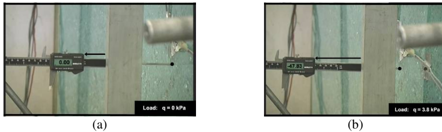
Figure 10: Broken laminated panel. Measured sag (a)→(b) under positive +3.8 kPa pressure.
