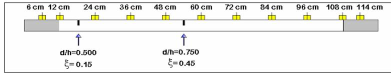
Figure 5: Crack and sensor positions along the beam span.
