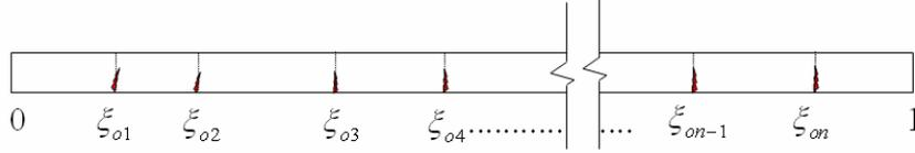
Figure 1: The beam segments between the ends and the cracked cross-sections.
