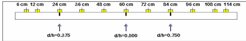
Figure 3: Crack and sensor positions along the beam span.
