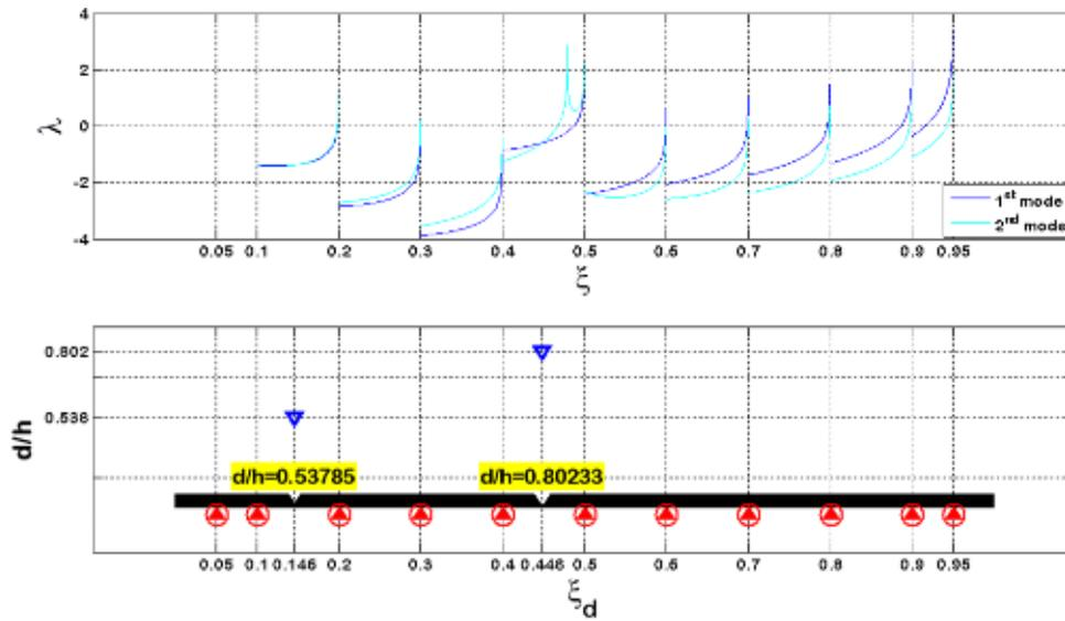
Figure 6: Identified damage intensities between each measurement position
