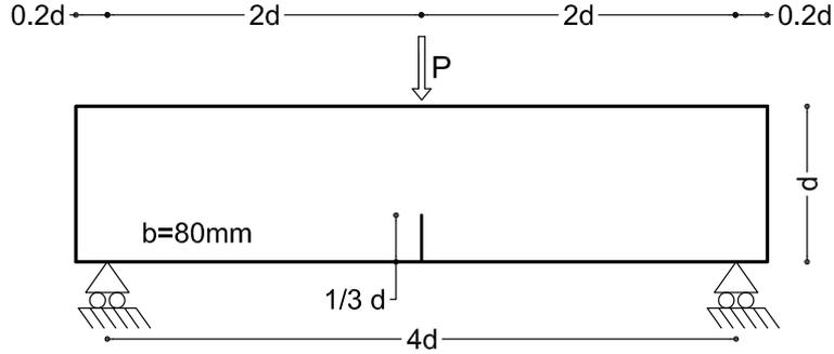
Figure 1: A three-point bending specimen.
