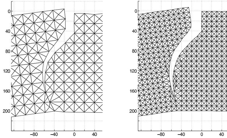
Figure 4: Detail of the deformed meshes in the region of the crack path: discretization 40x10 (L); discretization 80x20 (R).
