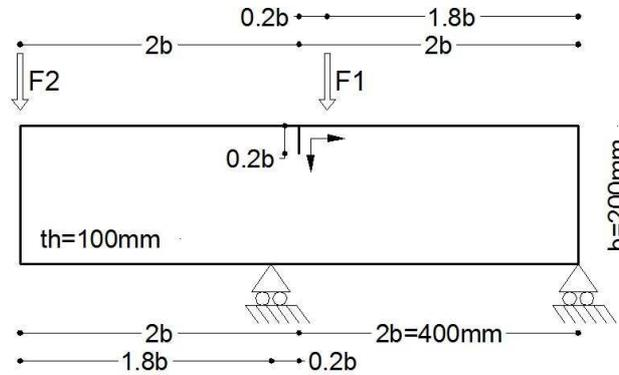
Figure 3: A four-point bending specimen.
