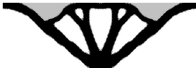
Figure 4: Optimal design for pressure load with the global constraint in Eqn. (7) 3 .
