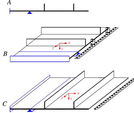
Fig. 4 A-B-C: two-dimensional representation of a typical one-dimensional input (A), in SAA approach (B) and BLT approach (C)
