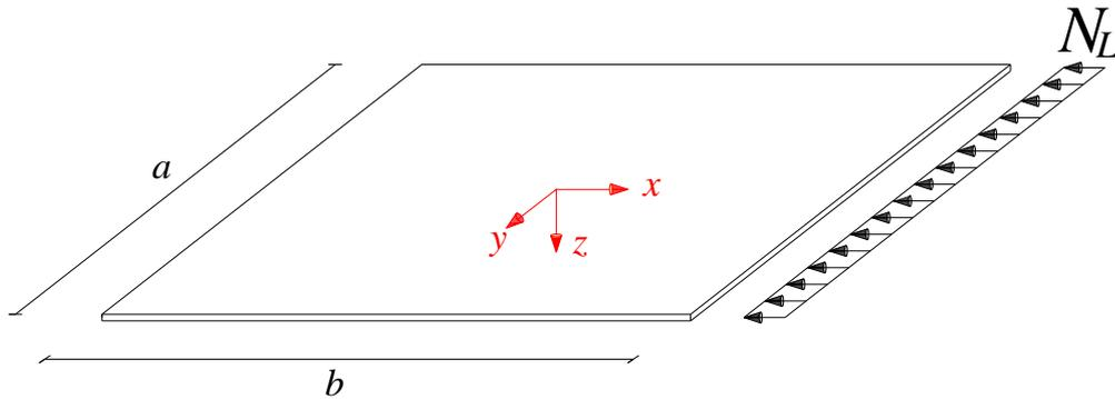
Fig. 1. Thin rectangular plate under in-plane load: dimension and reference frame
