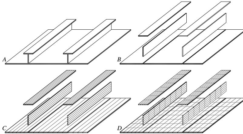
Fig. 2 A-B-C-D. (A) Typical stiffened plate and comparison between analytical (B), FSM (C) and FEM (D) required discretization
