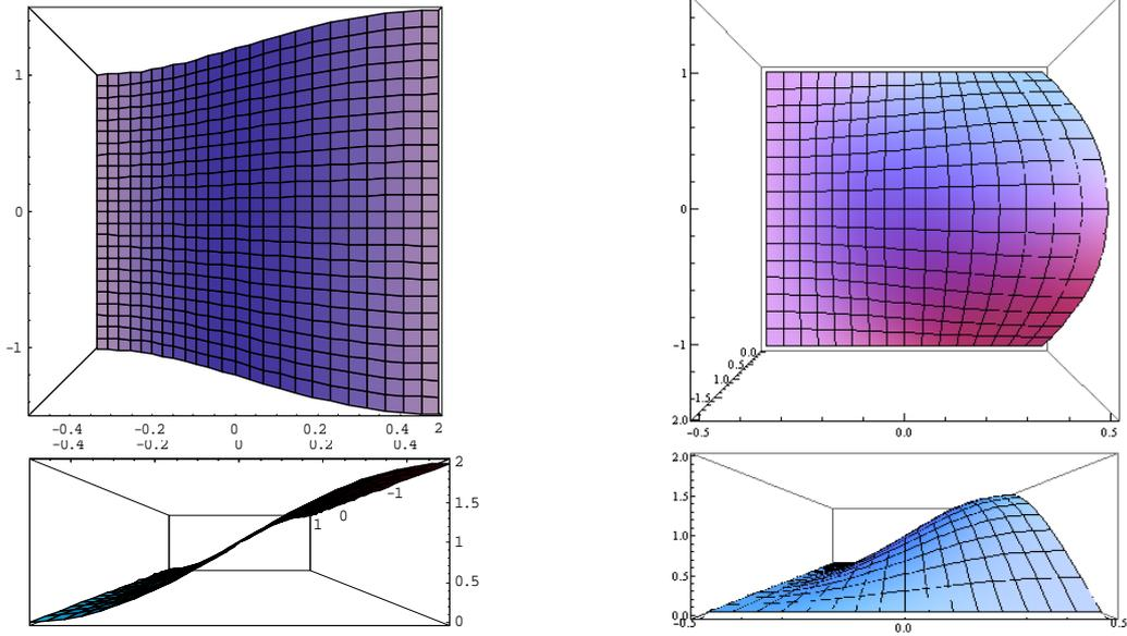
Fig 7: first mode of clamped-free plate of dimensions L and H, with BLT approach
