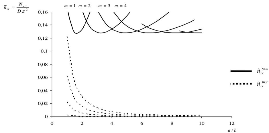
Fig. 6: Critical load of clamped-free plate via SAA approach and BLT approach
