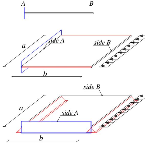
Fig. 5. Imposed boundary condition of a free plate (A) in BLT (B) and SAA (C) approach
