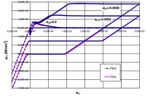
Figure 3: Mechanical response of the unit cell M2 subjected by the first loading history.
