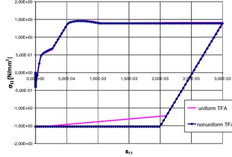
Figure 5: Mechanical response of the unit cell M2: comparison between TFA analyses.
