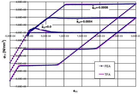
Figure 2: Mechanical response of the unit cell M1 subjected by the first loading history.
