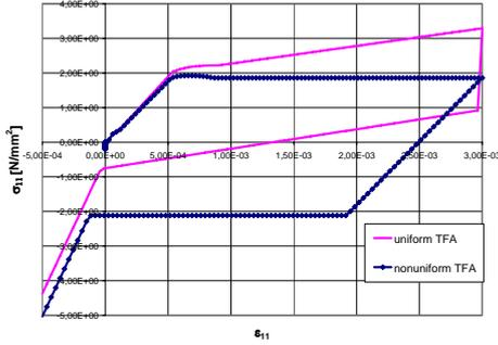
Figure 4: Mechanical response of the unit cell M1: comparison between TFA analyses.
