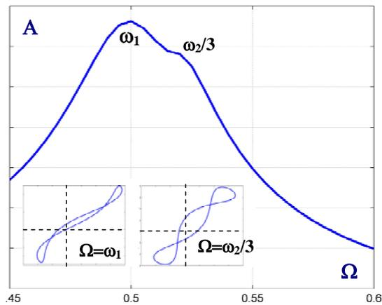
Figure 7. Frequency response curves and steady-state responses corresponding to  $\Omega=\omega_1$  and  $\Omega=\omega_2/3$  at  $\varepsilon=0.60$ . High damping.
