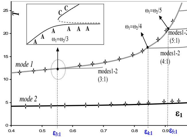
Figure 2 Period-damage plot of NLMs 1 and 2:  $(n:1)$  internal resonance.
