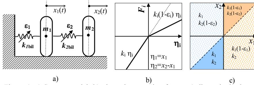
Figure 1. a) System model; b) piecewise restoring forces; c) discontinuity boundaries in the physical plane.
