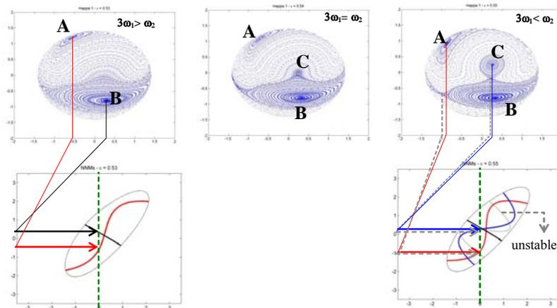
Figure 3. Cyclic-fold bifurcation caused by a  $(3:1)$  internal resonance around  $\varepsilon_{3:1}=0.54$
