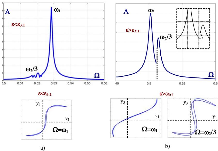
Figure 6. Frequency response curves and steady-state responses for  $\Omega=\omega_1$  and  $\Omega=\omega_2/3$  near  $\varepsilon_{3:1}=0.54$ . Low damping. a)  $\varepsilon=0.52$ ; b)  $\varepsilon=0.60$ .
