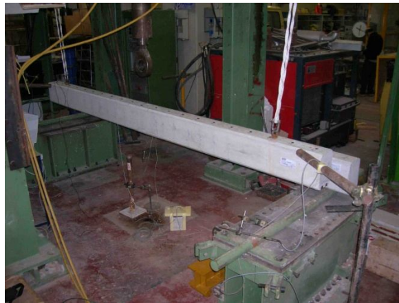
Figure 11: Dynamic tests of vibration on RC beam (B1) with free-free ends.
