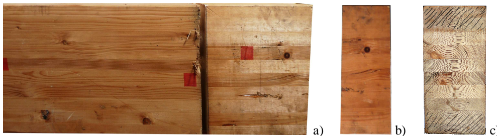
Figure 4: a) On-sale rectangular beam; b) piece from which the specimens have been obtained; c) cross section of the piece in b).
