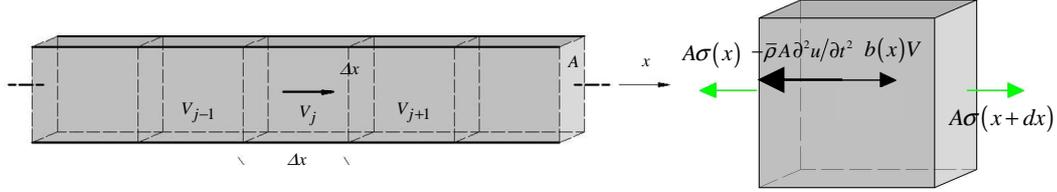
Figure 2: a) 1D model of viscoelastic bar; b) Equilibrium of 1D volume element
