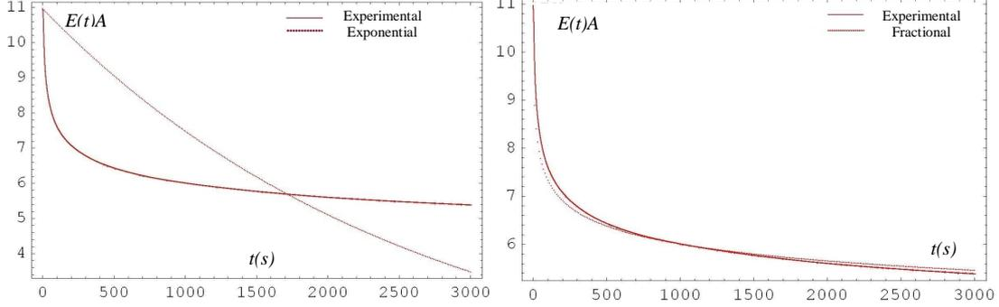
Figure 1: Static set-up on viscoelastic rubber: a) Continuous line experimental, dashed-line exponential best fit, b) Continuous line experimental, dashed fractional-power law best fit
