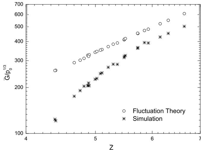
Figure 4: Comparison between theory and numerical simulation for the normalized shear modulus  $\bar{G}/p_0^{1/3}$
