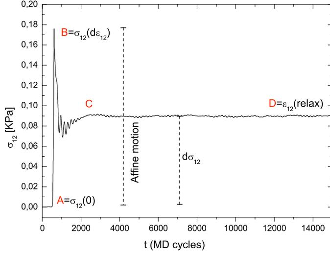
Figure 1: Numerical protocol for the calculation of the elastic response of the aggregate when an increment in shear is applied.
