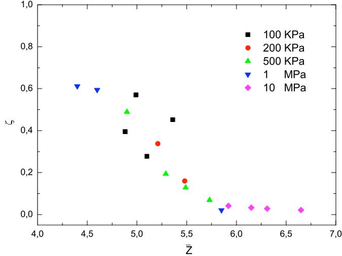
Figure 3: Variation of  $\zeta$  with  $\bar{Z}$  for increments in shear and compression.
