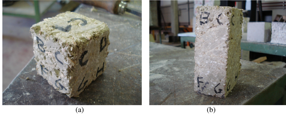
Figure 2. The specimens for the compression tests: a) cubic 50×50×50 cm, b) prismatic 45×58×112 cm.
