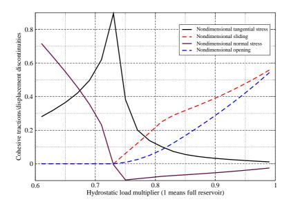
Figure 4: Tip response at 2 m from upstream side vs. load multiplier (pressurized fracture).
