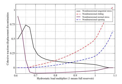
Figure 1: Tip response at 0.12 m from upstream side vs. load multiplier (dry fracture).
