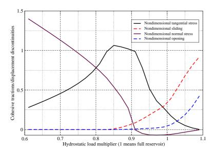
Figure 3: Tip response at 2 m from upstream side vs. load multiplier (dry fracture).
