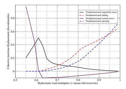
Figure 2: Tip response at 0.12 m from upstream side vs. load multiplier (pressurized fracture).
