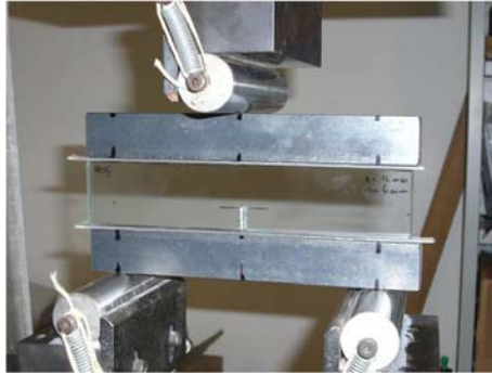
Figure 2.2 Sandwich beam apparatus used to naturally pre-crack the glass specimens.
