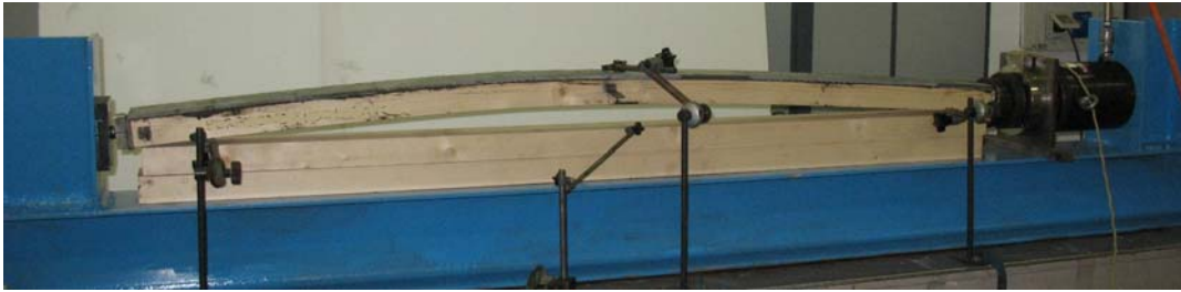
Figure 9: 300 mm tiles and adhesive 3: deflection higher than 50 mm.
