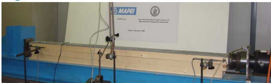
Figure 6: Test setup and a tested specimen reproducing tiled flooring.
