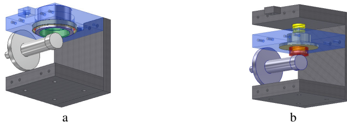
Figure 7: Two additional modules of the experimental apparatus with moving axis of the cam: rotating follower (a) and cam-follower coupling similar to the one used in i.c. engines (b).
