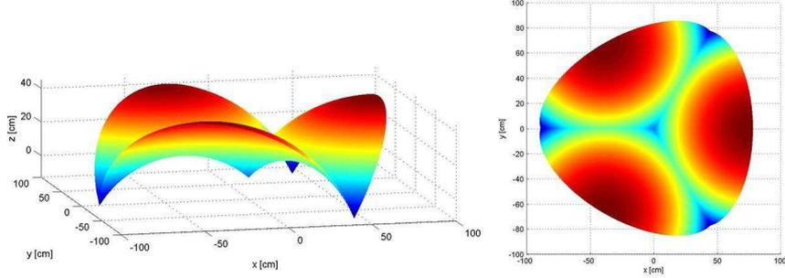
Figure 9: Two views of the lower frontier of the linear delta manipulator
