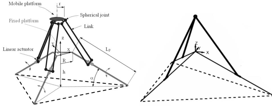
Figure 1: The 3dof parallel linear manipulator with its simplified model
