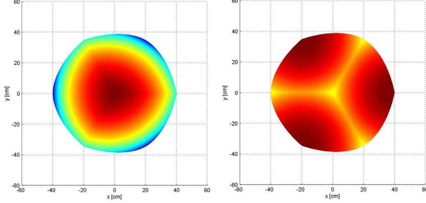
Figure 10: Upper and lower limit of the classic delta robot
