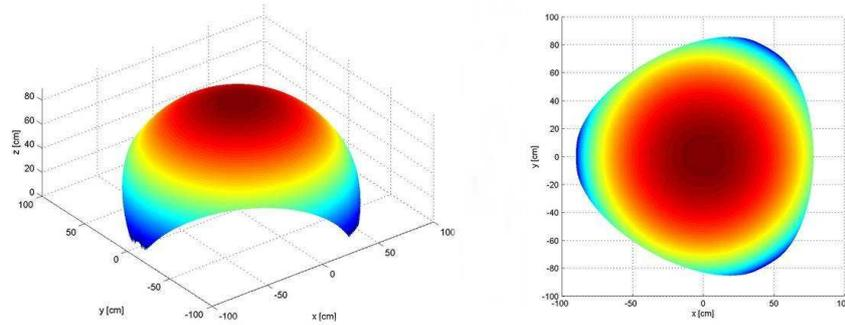
Figure 8: Two views of the upper frontier of the linear delta manipulator
