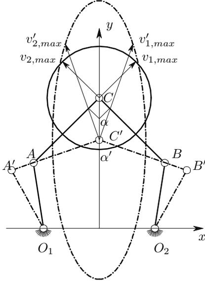
Figure 8: Ellipses of manipulability in velocity as function of manipulator configurations
