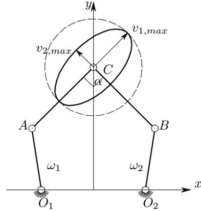
Figure 9: Ellipse of manipulability in velocity in an isotropic configuration when the motor is driven by two different motors
