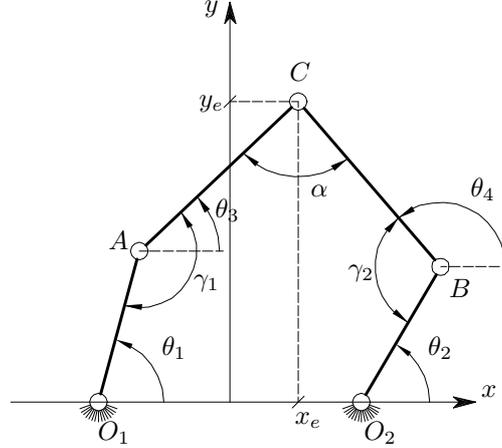
Figure 2: Layout of the robot
