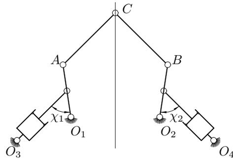
Figure 11: Planar manipulator driven by linear motors
