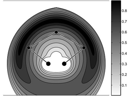
Figure 4: Values of the inverse of index  $I_3$  in the manipulator workspace
