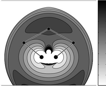
Figure 3: Values of index  $I_2$  in the manipulator workspace
