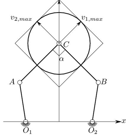
Figure 7: Ellipse of manipulability in velocity in an isotropic configuration
