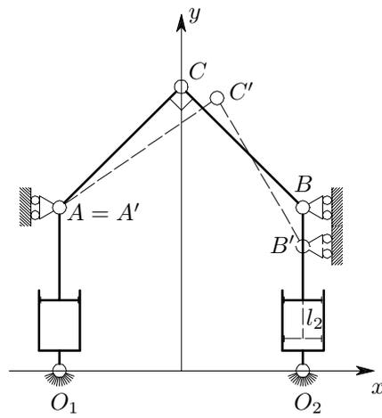
Figure 13: A planar 2dof manipulator driven by linear actuators characterized by drive system isotropy.
