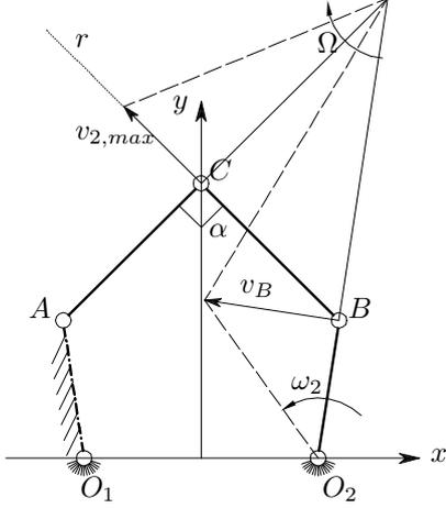
Figure 6: Maximum velocity along  $r$  direction
