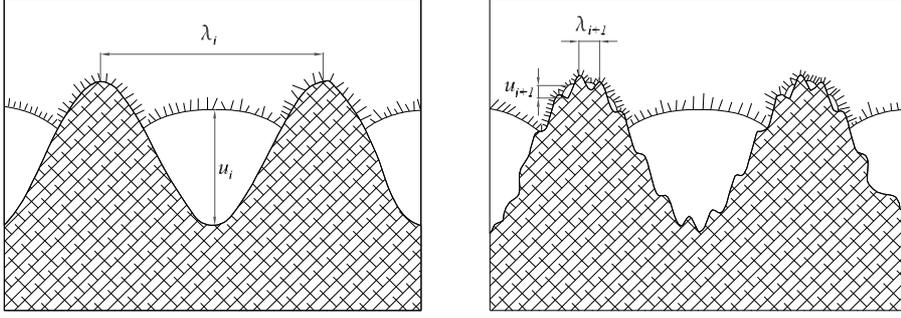
Figure 2: Sketch of a two-scale rough profile in contact with an elastic block. At scale  $i$  the voids have a width  $\lambda_i$  and height  $u_i$ , while at scale  $i + 1$  the voids have a width  $\lambda_{i+1}$  and height  $u_{i+1}$ . In three dimensional contact the voids have dimensions of order  $\lambda_i \times \lambda_i \times u_i$ . The picture is not in scale: according to theory of contact mechanics  $u \ll \lambda$ .
