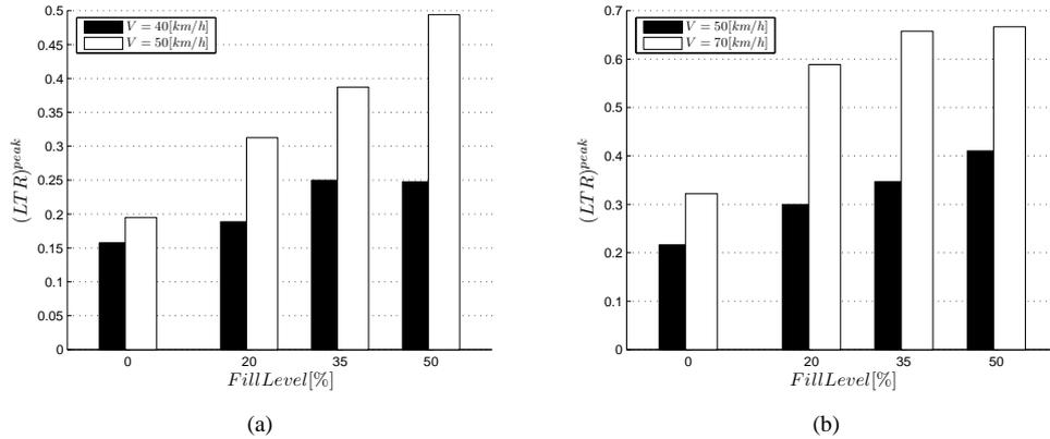
Figure 9: Predicted Load Transfer Ratio ( $LTR$ ) as function of the fill level for different values of constant longitudinal speed in (a) a double lane change and (b) roundabout. Measured steering angle is given as input.
