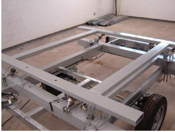
Figure 2: Six axis force measurement device: the lower frame is rigidly fixed to the trailer; the upper is mounted on six load cells. It measures forces and torques applied to the trailer.
