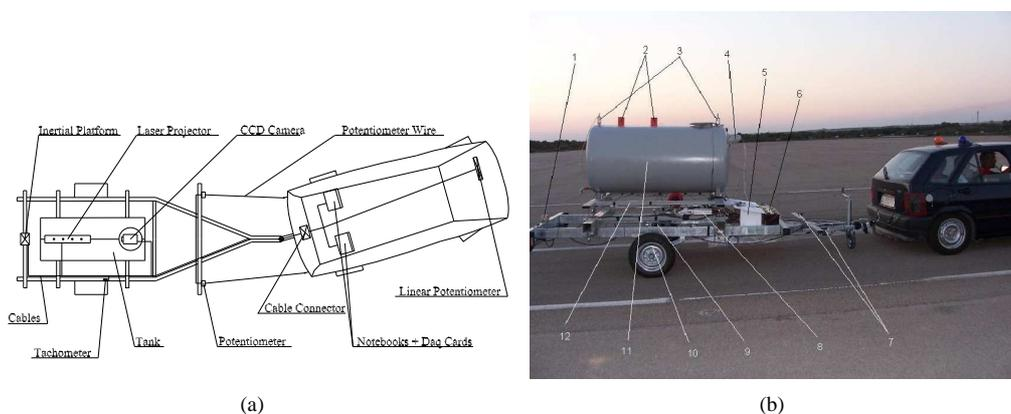
Figure 1: (a) Schematic of the experimental apparatus made of a car with tow hook and the instrumented trailer and (b) picture of the experimental trailer. 1 - Inertial Platform; 2 - Laser caps; 3 - Magnetostrictive float sensors; 4 - Camera; 5 - Cable connections and data acquisition device; 6 - Batteries; 7 - Linear wire potentiometers; 8 - AC/DC Converter; 9 - Steam potentiometer; 10 - Tachometer; 11 - Tank; 12 - Force device: upper frame.
