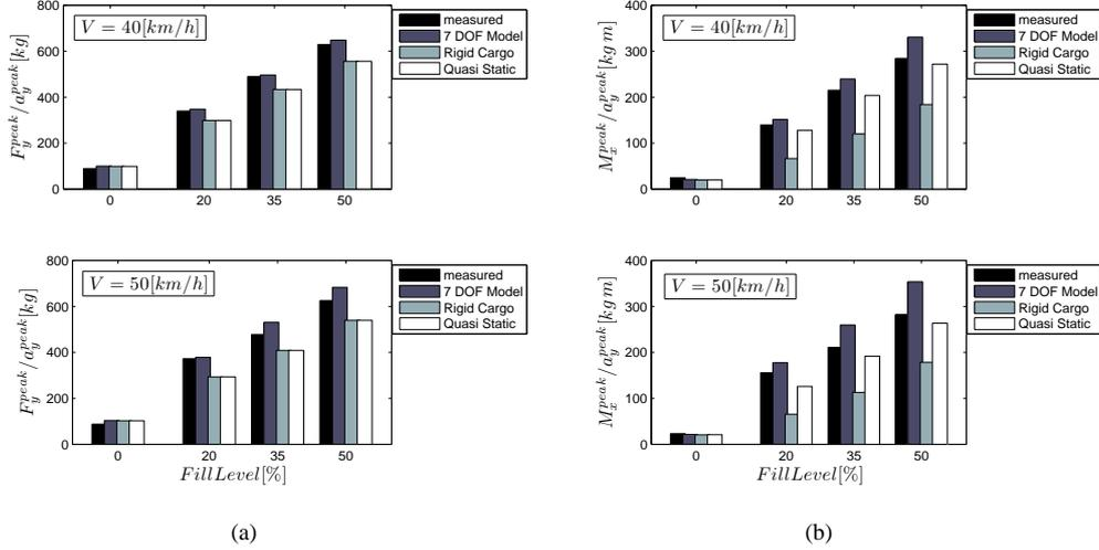
Figure 7: (a) Peak value of the lateral force  $F_y$  over the side acceleration  $a_y$  and (b) peak value of the roll moment  $M_x$  over the side acceleration  $a_y$  as a function of the fill level and for two different speeds (40 and 50 km/h) in a double lane change maneuver. Figure shows measurements and simulations results of three different mathematical models: full dynamical 7 DOF, quasi static and equivalent rigid cargo.
