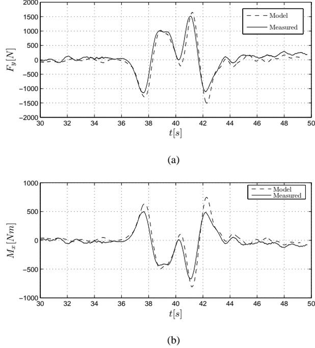
Figure 6: Time histories of (a) the lateral force  $F_y$  and (b) the roll moment  $M_x$ . Fill level is 35% and the longitudinal speed is 50 km/h.
