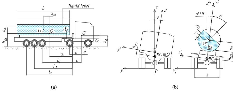
Figure 4: (a) Longitudinal and (b) transversal section of the truck-semitrailer
