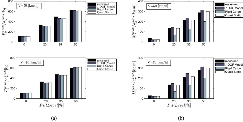
Figure 8: (a) Peak value of the lateral force  $F_y$  over the side acceleration  $a_y$  and (b) peak value of the roll moment  $M_x$  over the side acceleration  $a_y$  as functions of the fill level and for two different speeds (50 and 70 km/h) in a roundabout. Figure shows measurements and simulation results of three different mathematical models: full dynamical 7 DOF, quasi static and equivalent rigid cargo.
