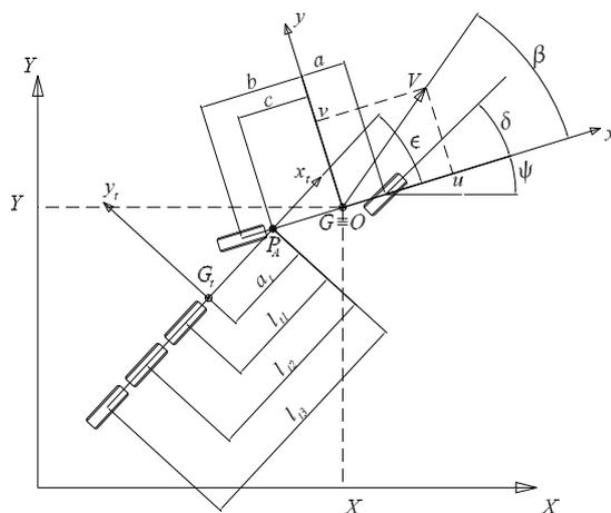
Figure 3: Reference systems and Lagrangian parameters
