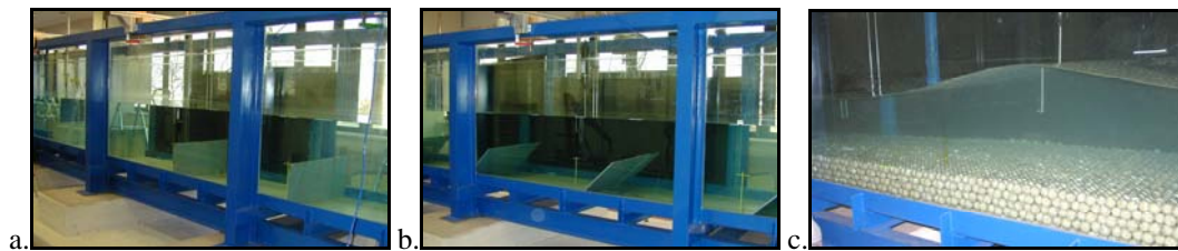
Figure 5: Seabed configurations with rough structures (a., b.) and porous bed (c.).
