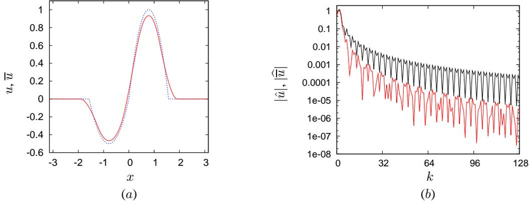
Figure 1: For a sample function  $u(x)$  (blue dashed line) its filtered one  $\bar{u}(x | \Delta)$  (red solid) with  $\Delta = \pi\sqrt{5}/10$  is drawn vs.  $x$  in (a), while in (b)  $|\hat{u}(k)|$  (black line) as well as  $|\hat{\bar{u}}(k | \Delta)|$  (red) are drawn vs.  $k$ .
