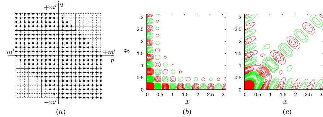
Figure 2: In (a), the wavenumber lattice  $\mathcal{L}_m$  is drawn. In (b, c) the level lines of the filters  $D_{m'}(x)D_{m'}(y)$  for  $m' = 10$  (min:  $-2.5$ , max:  $11.2$ ) and  $\mathcal{N}_c(x, y | m)$  (min:  $-1.2$ , max:  $8.3$ ) are drawn. Red lines indicate positive levels and green ones negative, with a step  $0.1$ .
